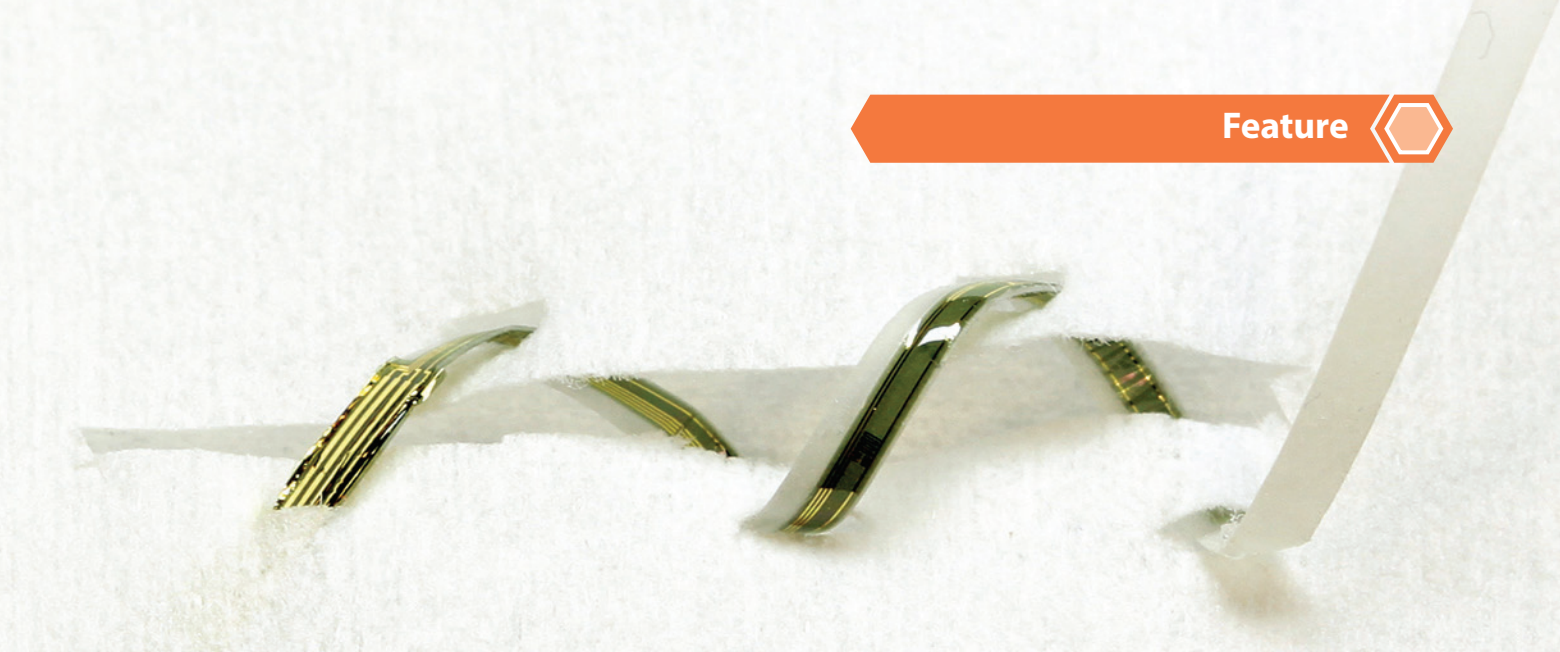
Optical image of a polymer-silicone suture strip after suturing. Credit: John Rogers, University of Illinois
